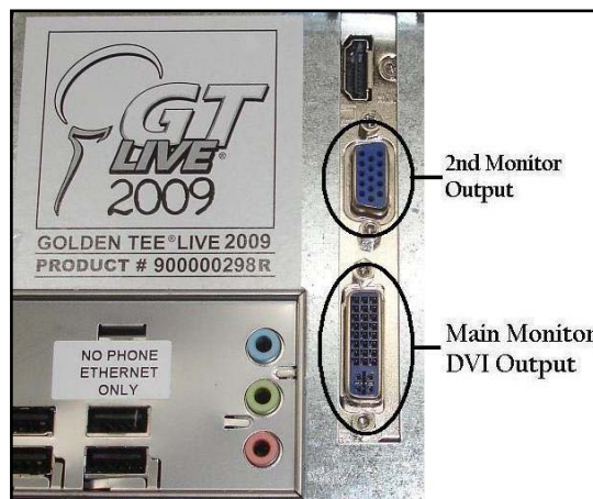
GT 2009 and 2010 have the same output configuration
