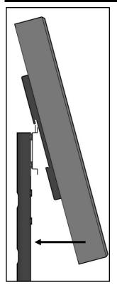
Use an assistant to carefully lift the HDTV and position it in front of the Monitor Bracket. Hook the two Vertical Brackets onto the top bar of the Horizontal Monitor Plate, then slowly swing the screen down and into place against the lower bar of the plate.
