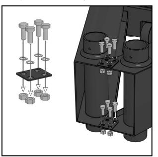
When installed properly, the brackets should be level with the ground, and flush against the backside of the cabinet to form a triangle.
