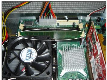
**Note**: If you have two or more memory modules, the system likely has sufficient memory, and a memory upgrade is not necessary. **Do not exceed 1 Gigabyte of memory**.
